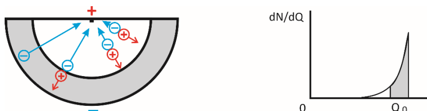
Fig. 4. Cross sectional view of a hemispherical detector showing the drift of electrons toward a positive “point” electrode and the resulting induced charge pulse. The majority of the induced pulse arises from electrons originating in the cross-hatched region of the hemisphere.
