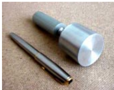
Fig. 2. Segmented detector with preamplifier.
