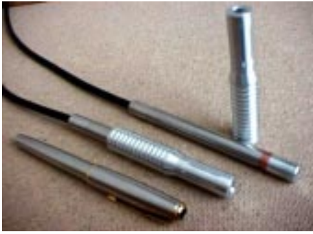
Fig14. Detection probes with Peltier element.
