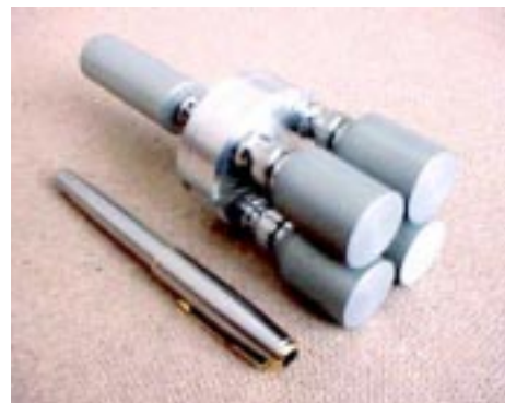
Fig. 8. Four element of assembled detector with connecting adapter and preamplifier.
