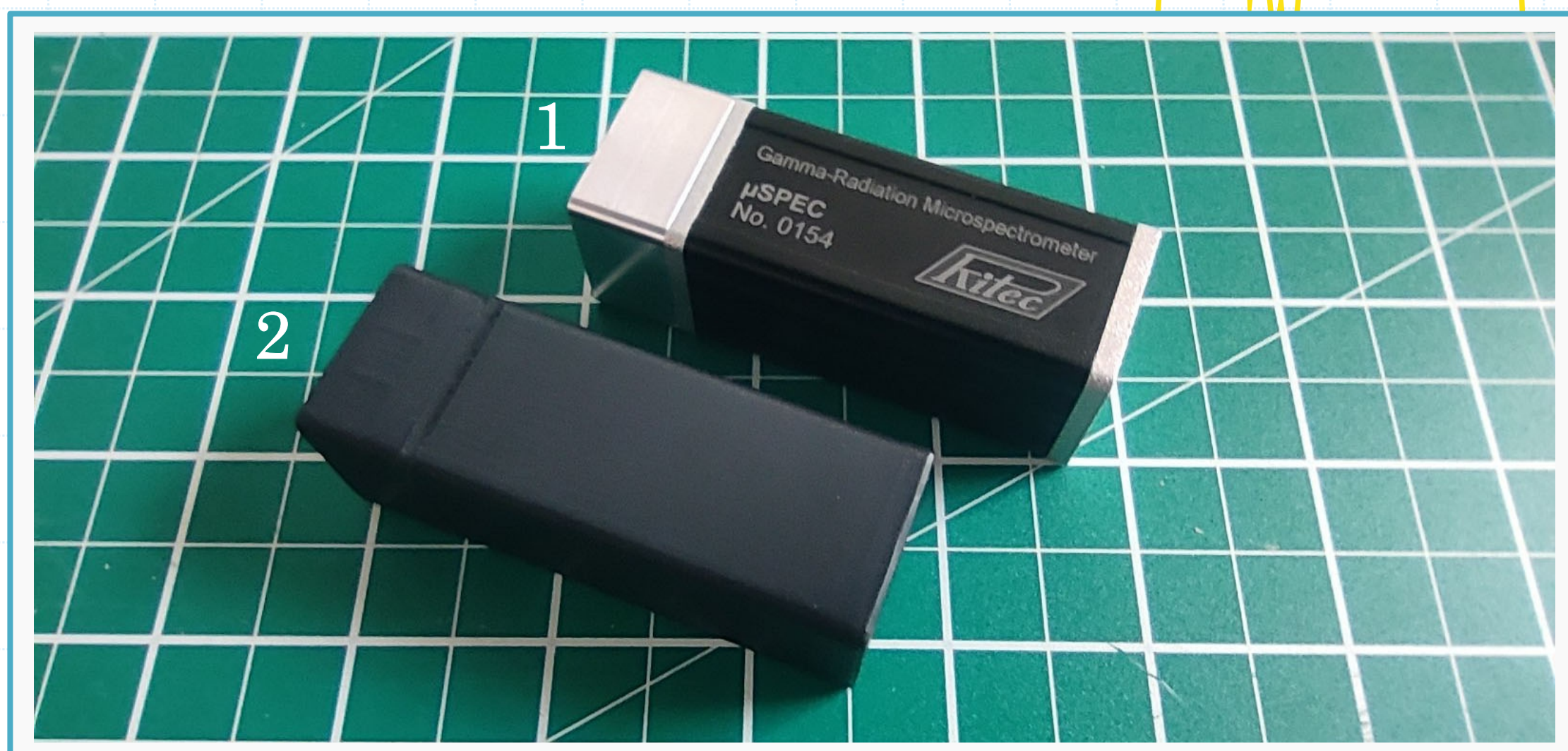
Micro spectrometers with a housing made of aluminum (1) and with a 3D printed (2).
