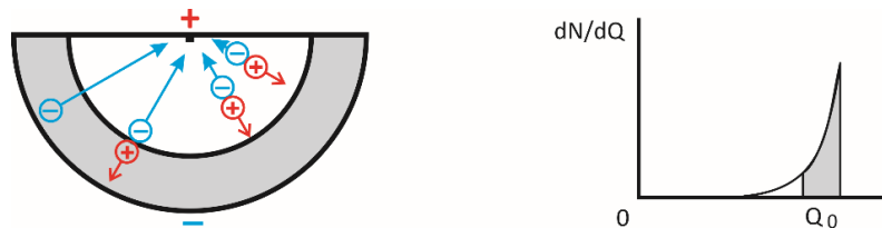
Fig. 8 – Cross sectional view of a hemispherical detector showing the drift of electrons toward a positive “point” electrode and the resulting induced charge pulse. The majority of the induced pulse arises from electrons originating in the cross-hatched region of the hemisphere.
